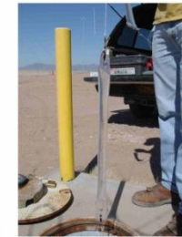
Collecting Samples with Diffusion Bags
